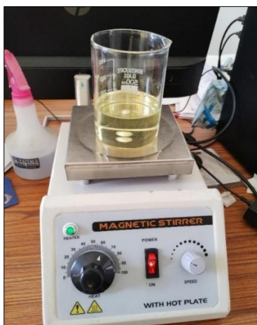
Fig 2.3: Mixing of catalyst and methanol with Chicken oil in magnetic stirrer
