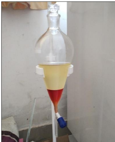
Fig 2.4: Separation of biodiesel (top layer) after alkaline esterification
